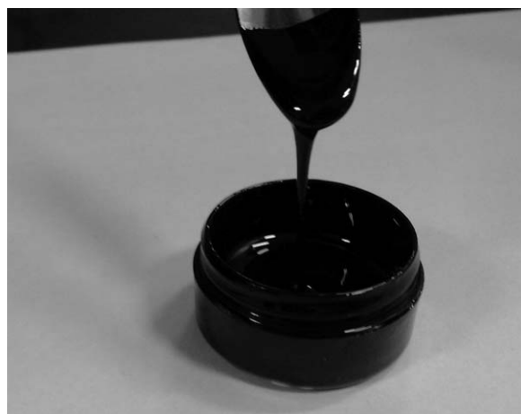
Figure 2. Picture of the liquid-like MWCNT derivative at room temperature.
