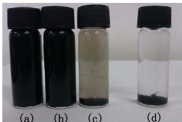
Figure 5. Solubility of liquid-like MWCNT derivative in (a) ethanol; (b) acetone; (c) water; and (d) solubility of MWCNTs in ethanol. [Color figure can be viewed in the online issue, which is available at wileyonlinelibrary.com .]
